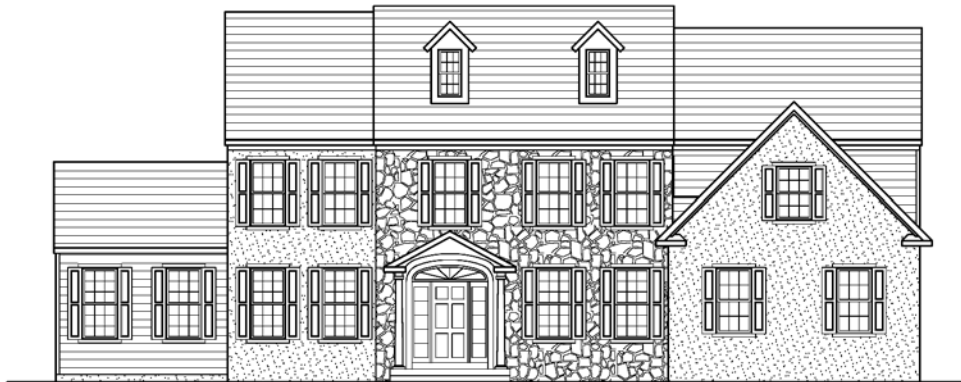
ELEVATION B: Stucco, Vinyl Siding & Stone Facade Shown With Optional Sunroom, Dormers, & Elliptical Front Pent Roof
