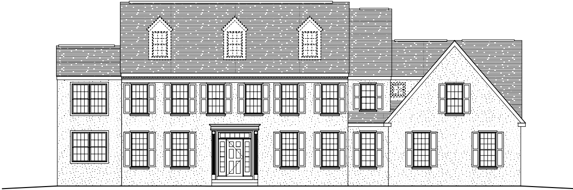
ELEVATION A: Standard Stucco Facade Shown With Optional Dormers & Window at Cricket
