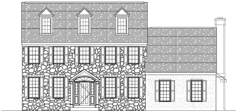
ELEVATION B: Stone & Vinyl Siding Facade Shown with Optional Dormers, Elliptical Pent Roof and Chimney
